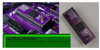
FNX6809 - MC6809 implemented in FPGA (a drop in replacement for the WDC65C02 for F256 Jr.)
