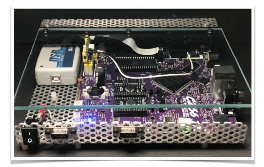
"Hinged roof, covered" - in this pic, joystick ports (front) are not yet wired but the JTAG interface is connected. The left side is open for easy access to the USB debug port and the *terasIC* FPGA blaster.
