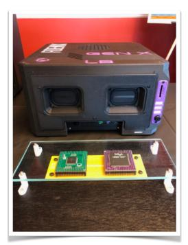
And with the addition of a second processor (such as a MC680x0 processor or an Intel i486/DX2), you can leverage a secondary power-up mode and transform your GEN X into a different machine, with a different OS and kernel, but with the same hardware capabilities and I/O including MIDI.
