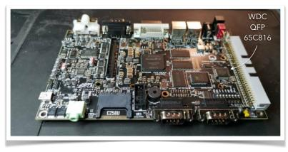
C256U - FMX heritage, WDC 65816 CPU @ 14 MHz. reduced chip count and lower cost
