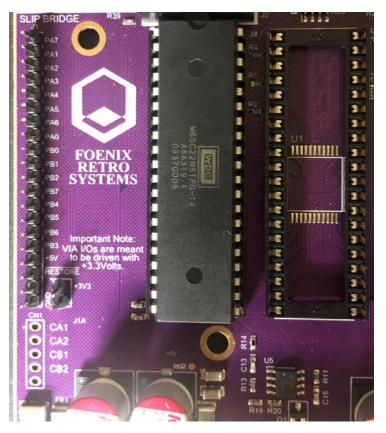
65C02 pulled to reveal this dev board's QFP footprint
