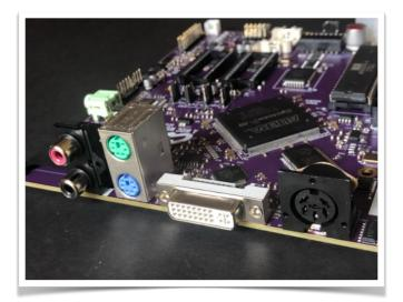
SD card (left, partially obscured), stereo audio line out, PS/2 mouse and keyboard; DVI-I video, and 6-pin DIN IEC (Commodore serial peripheral port)
