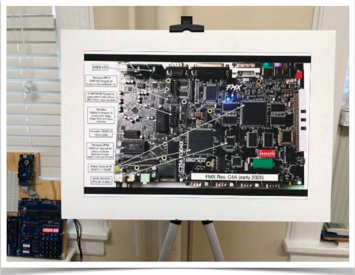
Picture of an early FMX board. Note the 40 pin PDIP based 65816 near the expansion connector on the right. All other boards\*, through the new GEN X utilize the QFP
