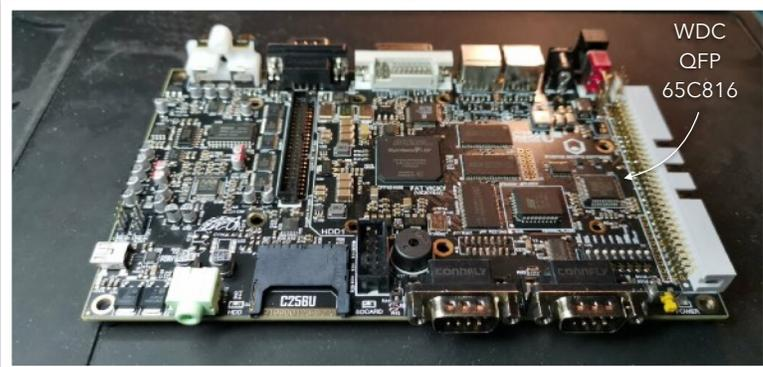
C256U - FMX heritage, WDC 65816 CPU @ 14 MHz. reduced chip count and lower cost
