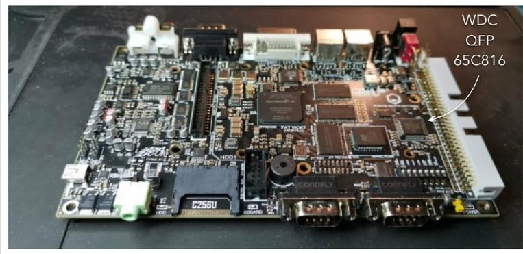
C256U - FMX heritage, WDC 65816 CPU @ 14 MHz. reduced chip count and lower cost
