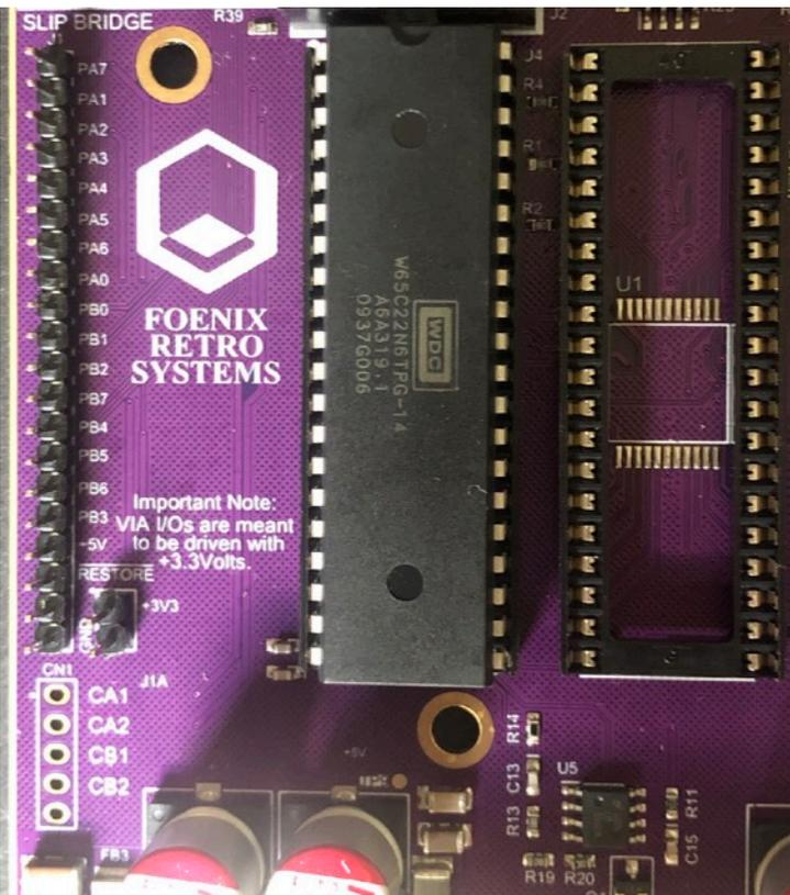
65C02 pulled to reveal this dev board's QFP footprint
