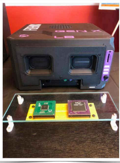
And with the addition of a second processor (such as a MC680x0 processor or an Intel i486/DX2), you can leverage a secondary power-up mode and transform your GEN X into a different machine, with a different OS and kernel, but with the same hardware capabilities and I/O including MIDI.
