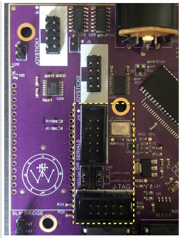
JTAG, jumpers, and headers for serial vs. "SLIP bridge"
