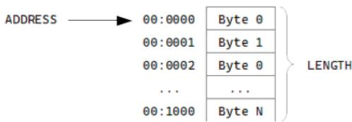
Figure 1: A linear (1D) memory block
