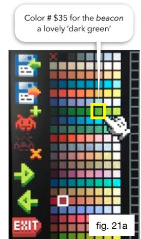
In last month's column, example "I01P11A.BAS" loaded LUT 0 with a full set of 255 colors which were identical to the default palette of the Foenix Sprite Editor. If you looked at the code, you saw that a FOR loop took a pile of values (768 of them) ranging from 0 to 255, and used SETCOLOR to build LUT 0.
