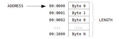
Figure 1: A linear (1D) memory block
