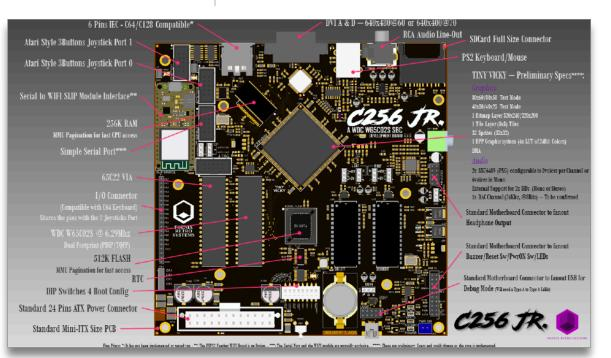
features as well, namely, a Serial to WIFI SLIP interface intended to get the platform on a local private net with a minimum of hassle.
