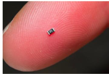
For scale: Stock photo of a '0603' 300nF capacitor
