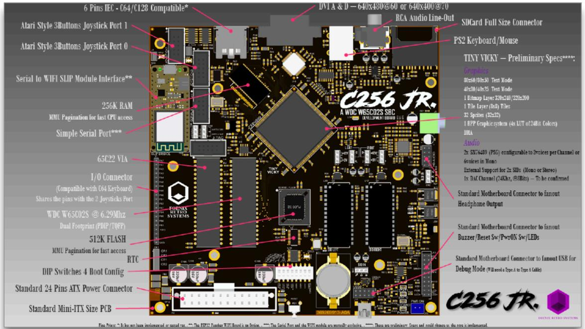
Something else unexpected: for the first time, a Foenix platform built to the Mini-ITX form factor with support for 24-pin ATX power; this will be familiar to PC and kit builders and opens the door to a world of options and customization, not the least of which could be a paring with cases such as the *My Retro Computer* Mini-ITX case (see [Kickstarter](#) campaign from earlier this month).
